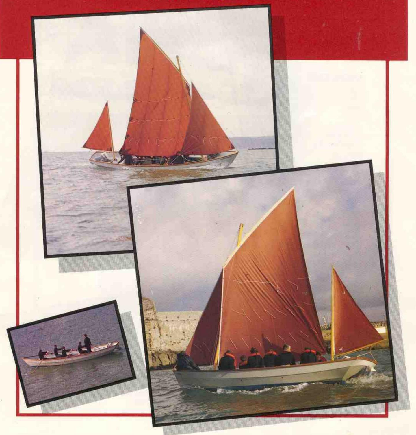
When sailing, the lug yawl rig is designed to give the crew plenty to do. Hence the reef points in the jib and three sets in the large mainsail.
