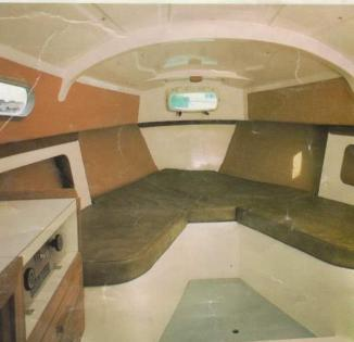
All boats are constructed of top quality glassfibre and polyester resin moulded under careful supervision. They are built in accordance with the current standards published by the Ship & Boat Builders' National Federation. Centreplate and rudder trunks are integral parts of hull mouldings.
