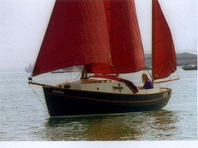
The original Drascombe Drifter was part of the Drascombe range designed by John Watkinson, a development of the Coaster which, amongst other refinements, incorporated a long centre keel with bilge plates to avoid the invasion of cabin space by a centreboard housing. A total of 110 Drifters had been built between 1977 to 1986 and although production stopped, any Drifters that come onto the secondhand
