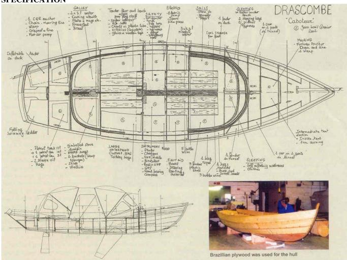
Hull & decks: wood epoxy.
